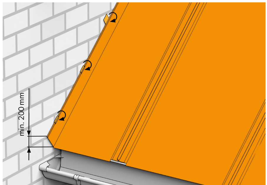
FIG.37 WALL FLASHING ASSEMBLY
