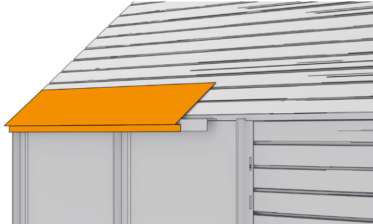
FIG.61 INSTALLATION OF PANELS ON THE ROOF SLOPE
