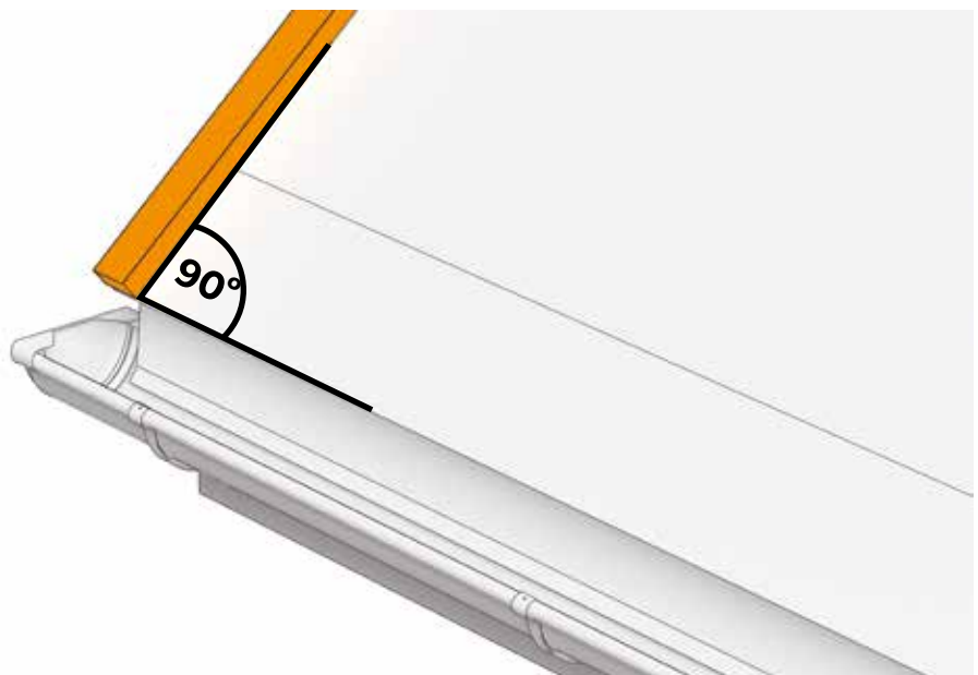
FIG. 10 WIND BRACE STRIP - ONE OF THE POSSIBLE SOLUTIONS
